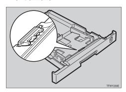
Reload paper with the print side up into the paper tray. While lifting the front side of the tray, insert the paper tray into the printer. Then push in until it stops.
